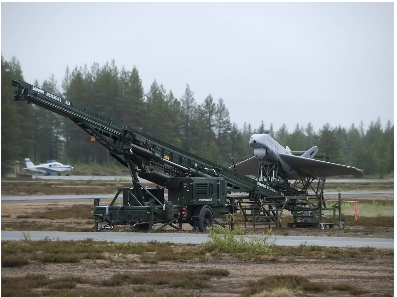
Sagem Défense Sécurité Sperwer-A ready for launch at RATUFC on a Robonic MC255LLR.
